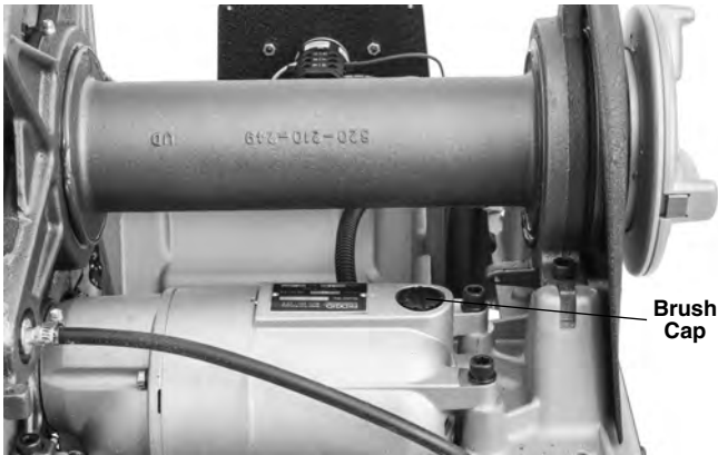
Figure 34 – Removing Motor Cover/Changing Brushes
