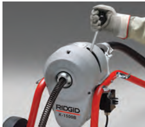
Release handle, cable stops instantly.
