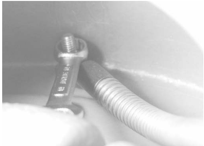
Figure 14 – Removing Pigtail Anchoring Bolt
